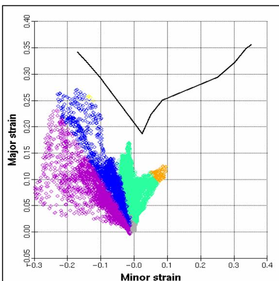
Fig. 5. Formability assessment of an automotive part with (a) #3 sheet and (b) #4 sheet.
