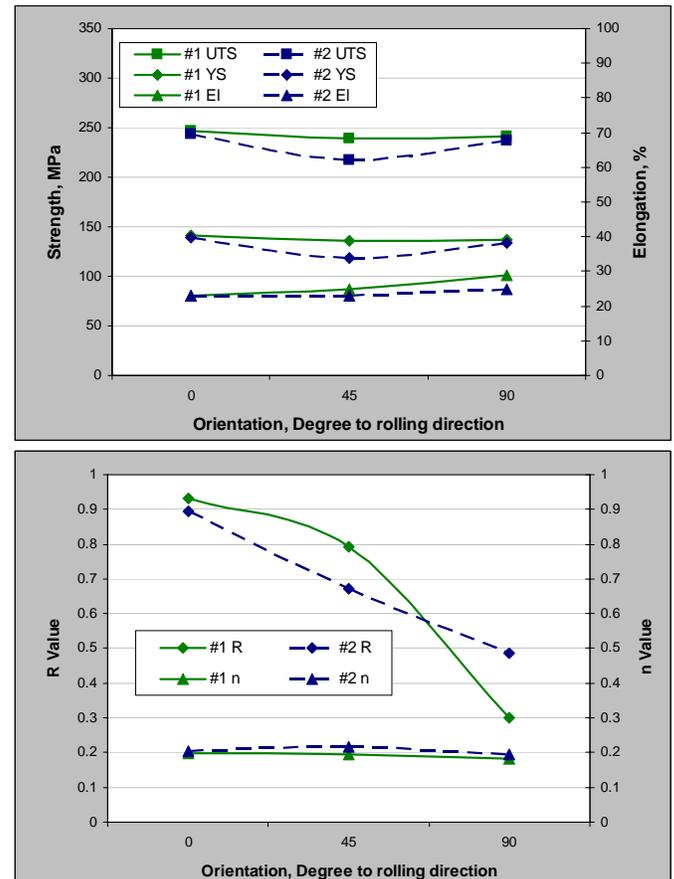
Fig. 2. Effect of Fe on tensile plastic behavior showing (a) strength and ductility and (b) anisotropy and work hardening.
