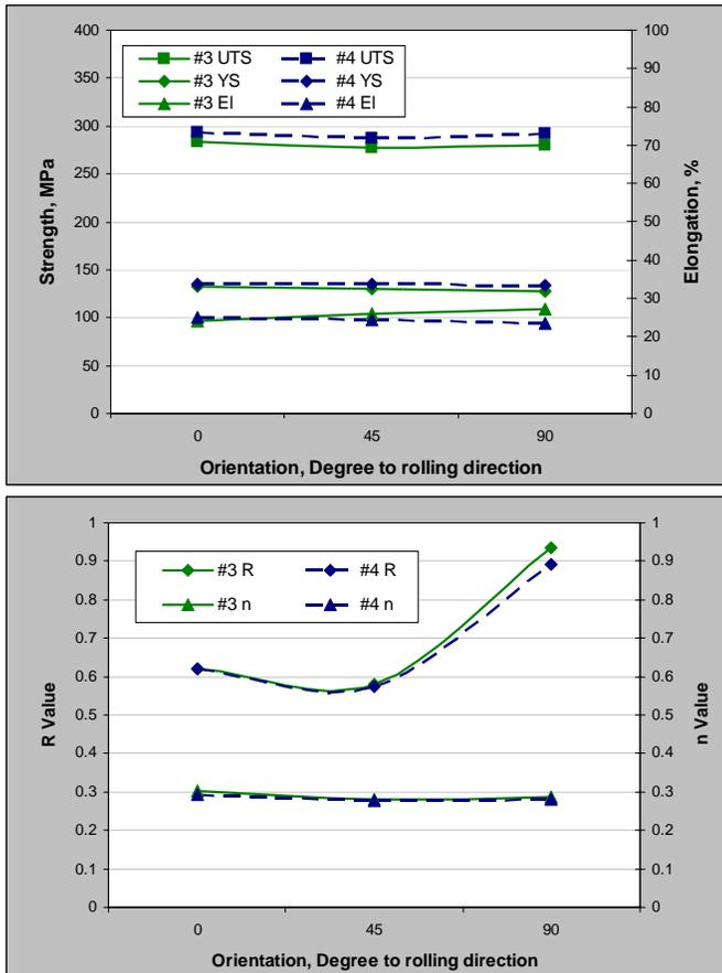
Fig. 3. Effect of Mn on tensile plastic behavior showing (a) strength and ductility and (b) anisotropy and work hardening.
