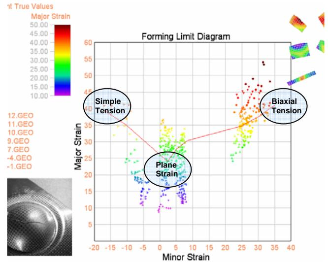
Fig. 1. Representative forming limit diagram.
