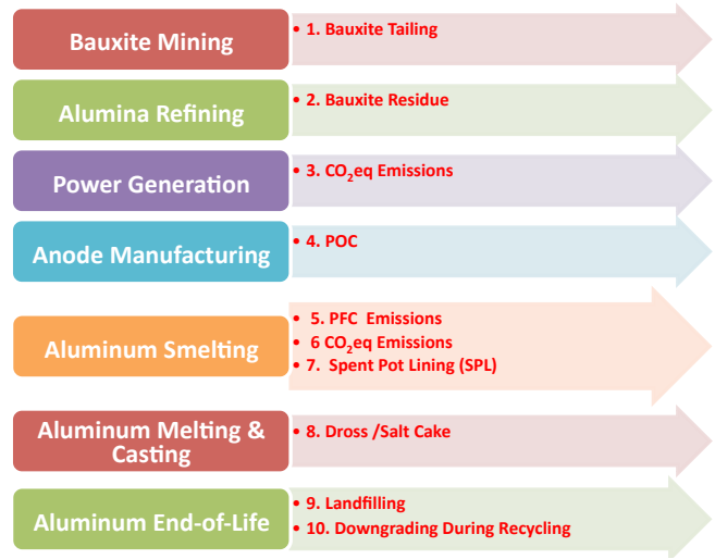
Figure 1. Aluminum production processes and their carbon and by-product emissions.
